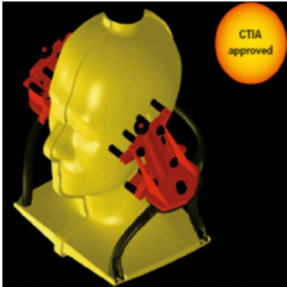
SAM Phantom. The red devices are clamps to hold the cellphone in a specified location. "CTIA" is the Cellular Telecommunications Industry Association. Source: Speag Phantom Product Flyer.
