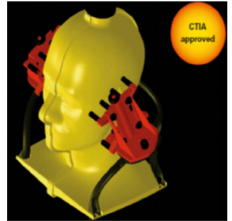
SAM Phantom. The red devices are clamps to hold the cellphone in a specified location. 'CTIA' is the Cellular Telecommunications Industry Association. Source: Speag Phantom Product Flyer.
